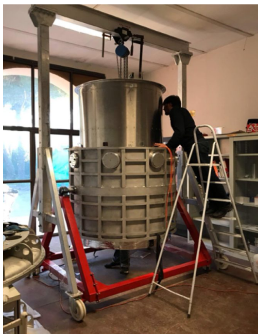
Figure 3: 40 K shield mounting in cryostat
