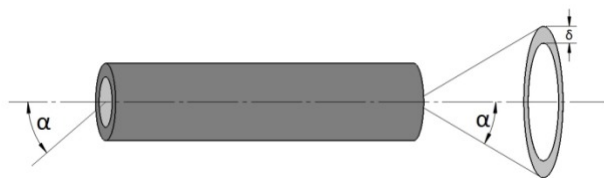
Figure 3- Condition observed in a fiber fed with a beam having no divergence, i.e. the input beam has NA=0 . Incorrect aiming with respect to the optical axis of the fiber results in a ring of light at the input angle.
