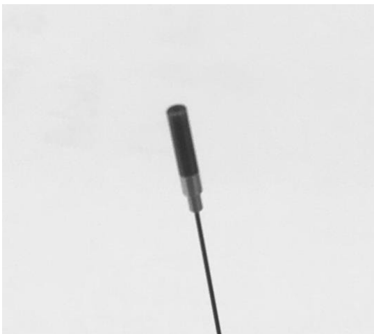
Figure 1- Photograph of a Zirconia ferrule with a fiber inserted.
