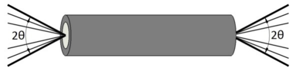
Figure 4- Condition observed in a fiber fed with a cone of light. In an ideal optical fiber, without any kind of FRD, the output reproduces exactly the same cone of light applied at the input.
