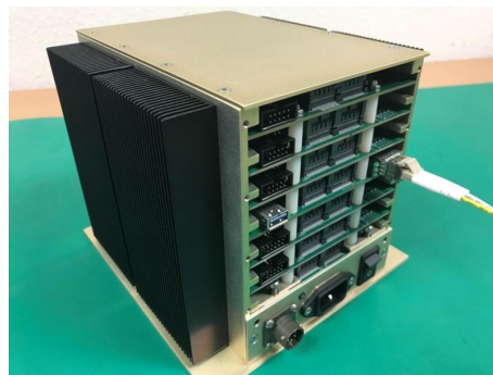
Figure 2. An example of an ARC box; similar enclosures will be attached to the side of the science cryostat and will house detector control electronics.
