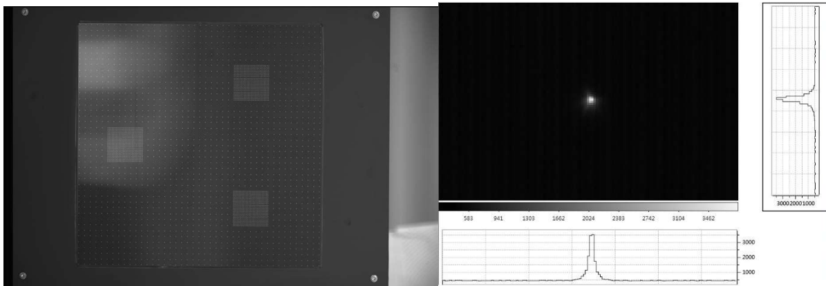
Figure 6. The pin hole mask image taken by MCS with the whole system tilted to the horizontal direction (left). The close view of the MCS image spot and the psf profiles (right)
