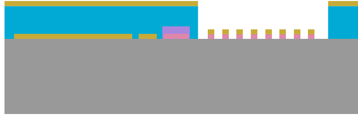
Figure 4. A diagram of the layer stack. First, the 20nm TiN layer (magenta) is deposited and patterned to define the KIDs. Next silicon oxide (purple) is deposited to protect the TiN inductors from being etched or damaged by future processing. The first niobium (gold) layer is then deposited and patterned. The 0.5 \mu\text{m} silicon nitride dielectric (light blue) and niobium ground plane are deposited, and both are then patterned and etched in the same step, exposing the capacitors of the KIDs and the antenna slots.
