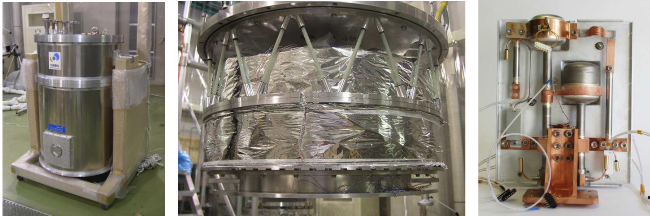
Figure 8: Z-Spec cryogenics. The left photo is an exterior view of the cryostat. The drum head mounting structure of the helium stage is seen in the middle. The closed-cycle ^3\text{He} / ^4\text{He} fridge is shown on the right. The pots are shown; the pumps are on the opposite side.
