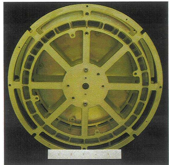
Figure 9. Two spiral lenses that have been tested at the XACT facility in Palermo. Their plastic ribbons are coated with an evaporated layer of Au. Better results will be obtained when they are replaced with W sputtered ribbons.
