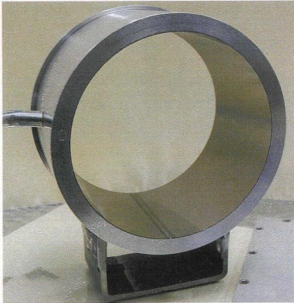
Figure 6. A 156 mm diameter vacuum mandrel mounted with a W coated PET shell. The joint is at the bottom.
