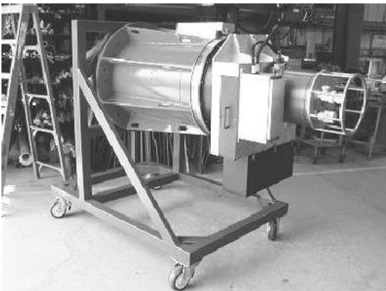
Figure 1: The SOAR Optical Imager. The interface to the telescope is the left-most flange of the braced tubular structure. The latter houses the two prisms of the atmospheric dispersion corrector. At its right-hand end is the rotator, which supports all the hardware to its right, plus the focal reducer optics. To the right of the rotator is found the filter, guider, and shutter box, to which is mounted the liquid-nitrogen cooled dewar, with a SDSU-2 (Leach) CCD Controller in front. Not shown in this picture is a second SDSU-2 Controller that is mounted behind the dewar, the external parts of the guider assembly, or the cable wrap assembly.
