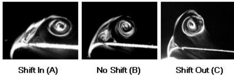
Fig. 2. Primary vortex shift in and shift out on the starboard side of the wind tunnel model.
