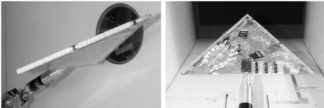
Fig. 8. Integrated MEMS sensors and actuators mounted on the wind tunnel model.
