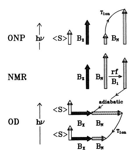
Fig. 2. Vector picture of time-sequenced optical nuclear magnetic resonance. The three processes of optical nuclear polarization (ONP), nuclear magnetic resonance (NMR) and optical detection (OD) occur in separate intervals and thus sensitivity and resolution can be simultaneously
