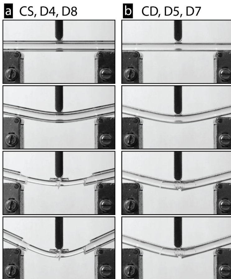
Figure S1. Flexure tests of struts with outer diameters 7 mm and 8 mm. Exemplary failures for outer diameters 8 mm (a) and 7 mm (b) are shown, which correspond to the load-displacement curves shown in Figure 2c and Figure 2c, respectively. The behavior is similar to the one of the CSS strut in Figure 2a: upon occurrence of the first crack, the shell fails completely and the core is capable of continuing to bear load until its own fracture strain is reached.
