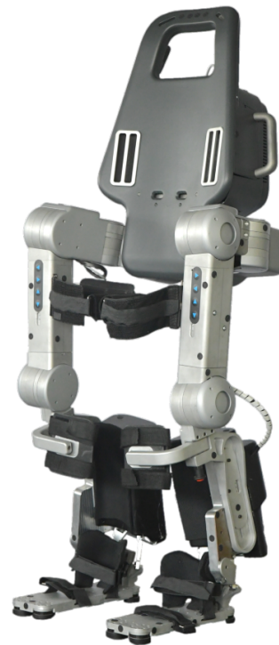
Fig. 1: ATALANTE: An exoskeleton designed by Wandercraft for people with paraplegia.
