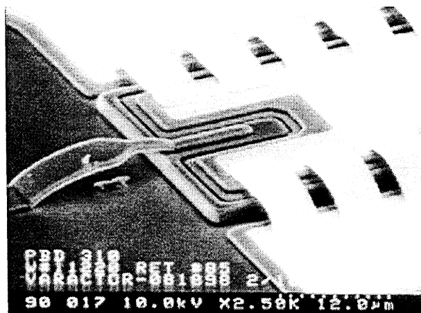
Figure 3 SEM of a rectangular anode Schottky diode and air bridge made at JPL.
