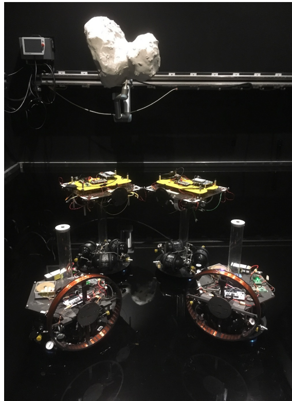
Fig. 1: Caltech’s Spacecraft Simulator Facility and Four M-STARs with the Two Docking Systems
