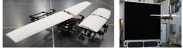
(a) Prototype VTOL with wing and tilt-rotor (b) Fan-array wind tunnel Fig. 7. Functional prototype winged VTOL flying in wind field generated by a fan-array wind tunnel, provided by Dr. Mory Gharib's group
