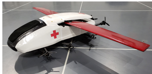
Fig. 1. Caltech’s VTOL flying ambulance (1/5 scale) that includes distributed electric propulsion, tilt-able rear rotors and a main wing.
