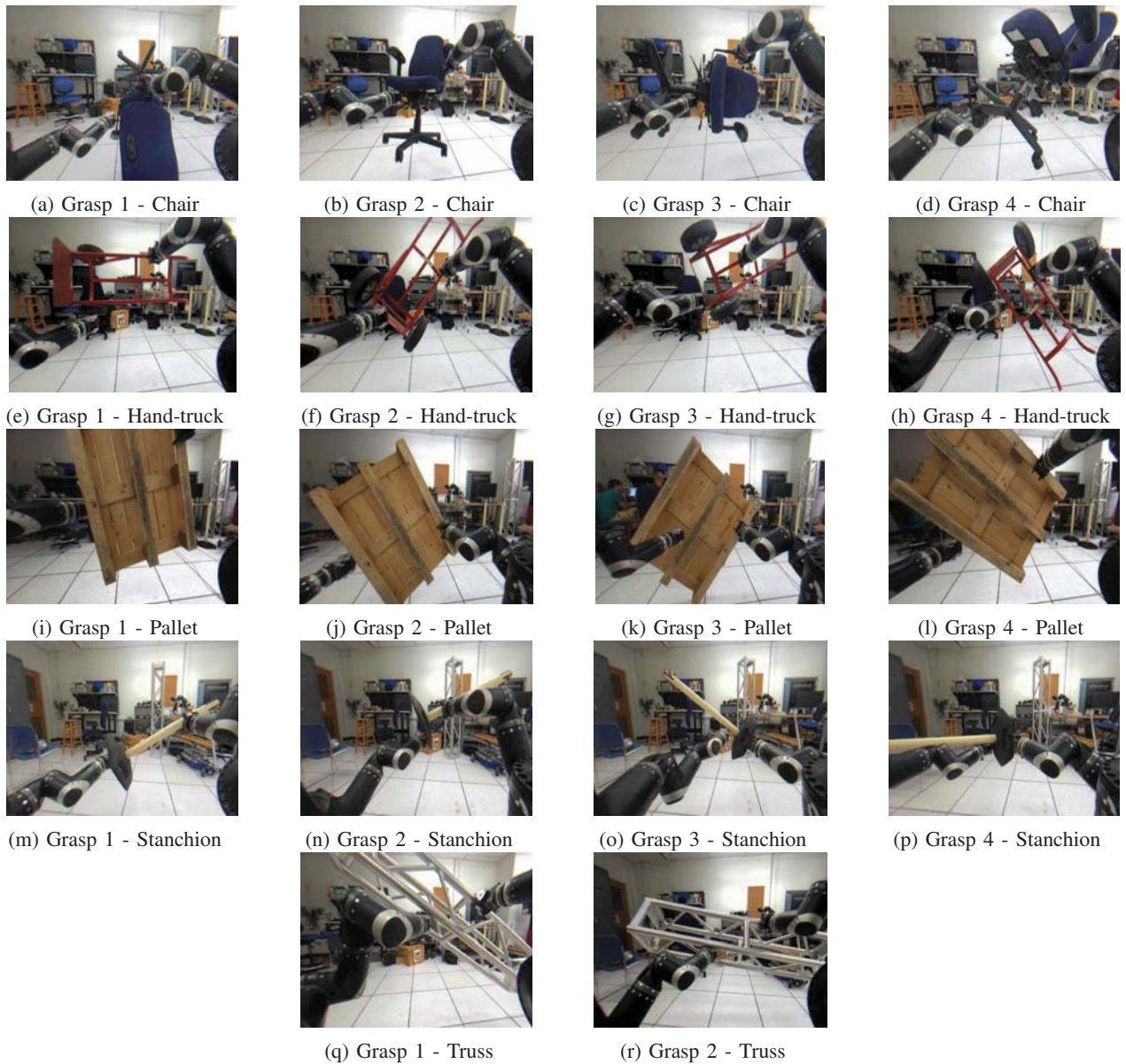
Fig. 7: Ending postures of an auto-adaptive dual arm behavior given different operator-specified initial grasp locations. The results are shown for a chair (25 kg), hand-truck(14.6 kg), pallet(14.2 kg), stanchion (7.6 kg) and truss (17.2 kg).
