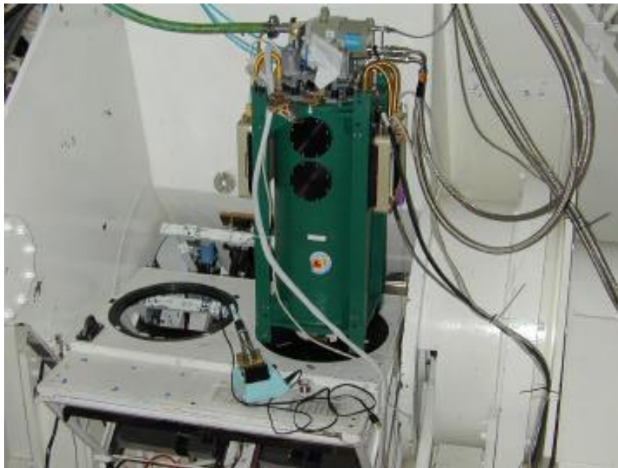
Figure 7. FIBRE in place on the Cassegrain relay focus of the Caltech Submillimeter Observatory on Mauna Kea, Hawai'i.
