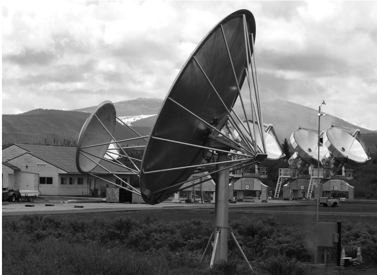
Figure 3: ATA antenna with existing BIMA dishes in background. BIMA is combining with the Caltech Millimeter-Wavelength Array and relocating to the Owen's Valley, CA area (Credit Seth Shostak).
