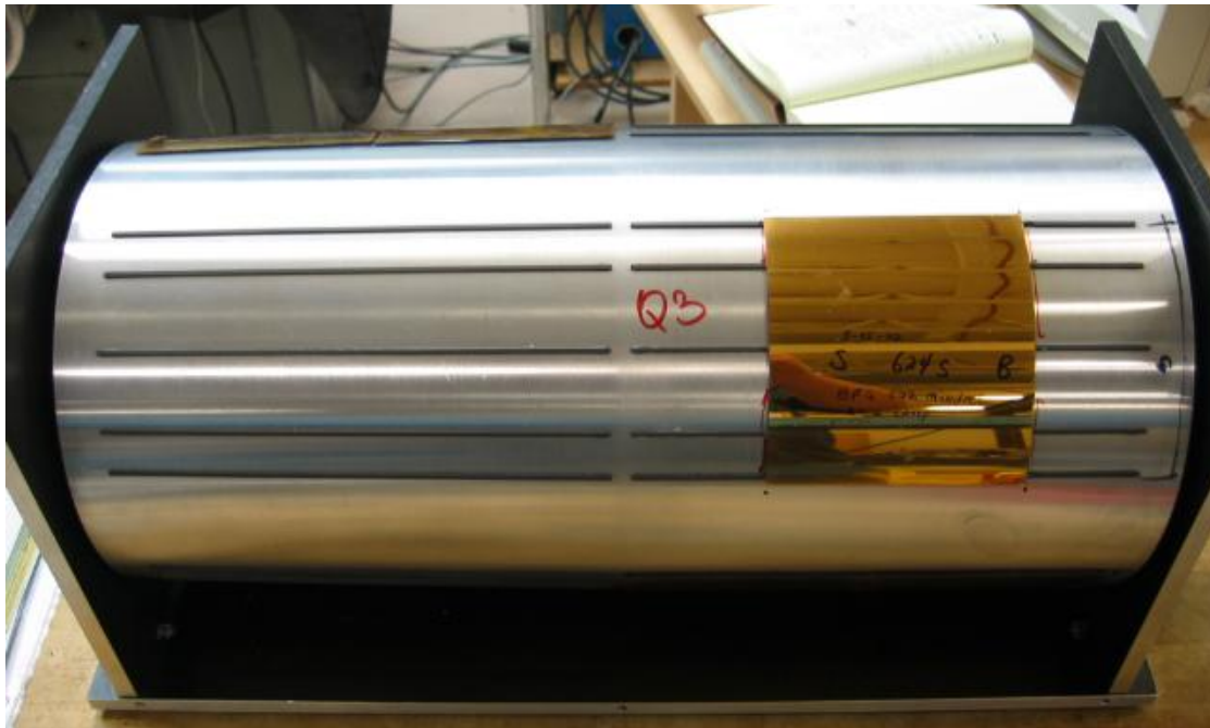
Figure 5: Con-X1 eGlass segment epoxied to 5 graphite spacers on the titanium mandrel.
