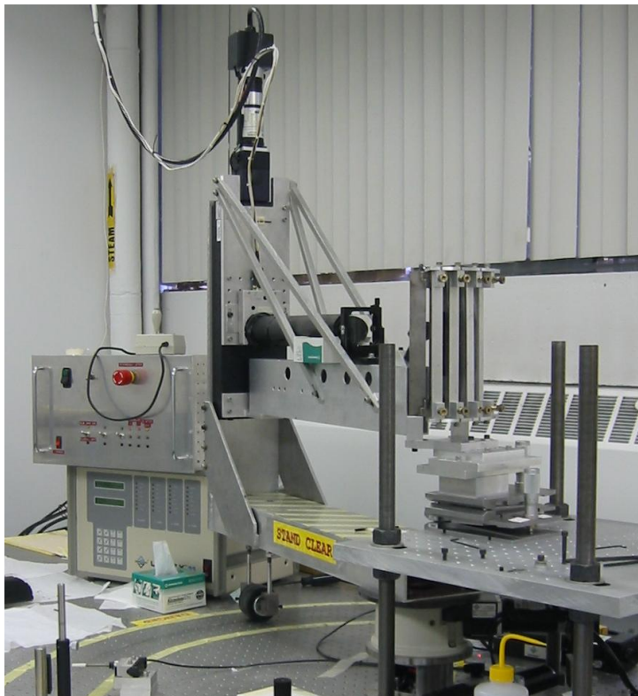
Figure 8: tGlass mounted in a surrogate mount on the laser reflectometer.
