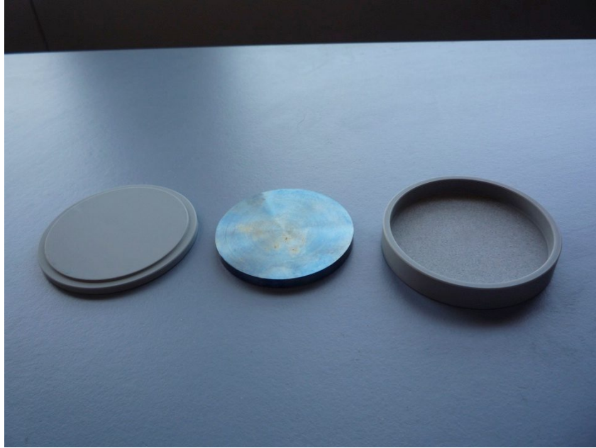
Figure 11 Steel disk and the ceramic enclosure we use to mask its glowing in the VIS
