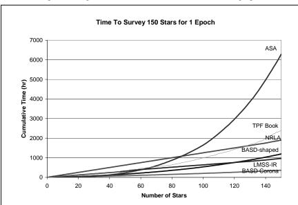
Figure 1. The cumulative time to search the habitable zones around a sample of 150 stars (1 epoch) is shown for 6 different architectures. The ASA performance could be improved with the implementation of a deformable mirror to further reduce scattered light.
