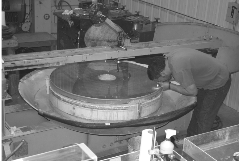
Figure 4: FIREBALL 1.2m diameter Siderostat mirror undergoing testing at Optical Mechanics, Inc.
