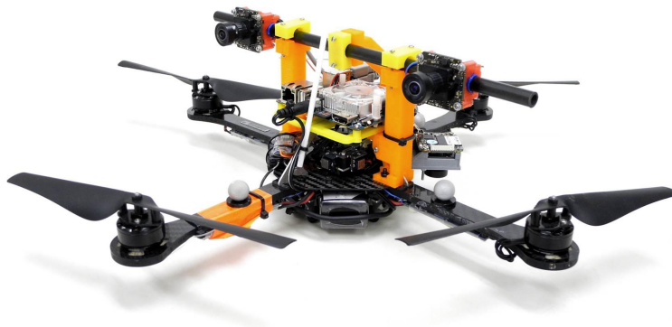
Figure 3: Asctec Hummingbird with stereo camera head and Odroid XU4 flight computer.
