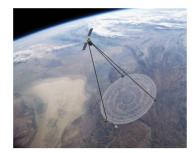
Figure 1. DARPA MOIRE concept shown conducting Earth observation
