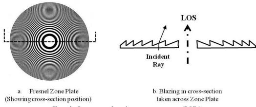
Figure 3. Components of membrane entrance aperture (DOE 1) Illumination incident along line-of-sight (LOS<sup>†</sup>)
