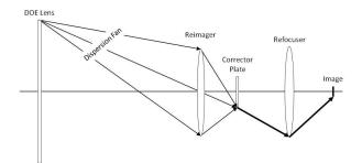
Figure 10. Representative diffractive telescope diagram
