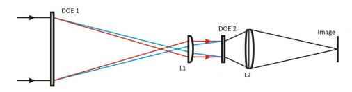
Figure 2. Nominal membrane telescope configuration (following Andersen<sup>4</sup>)
