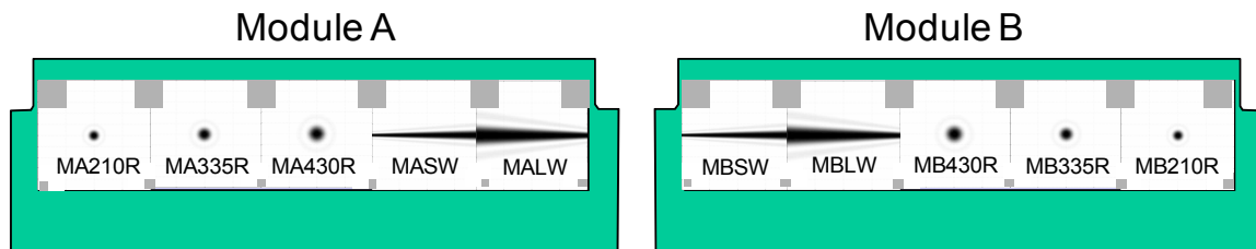
Figure 1. Occulting masks in the two NIRCam Modules
