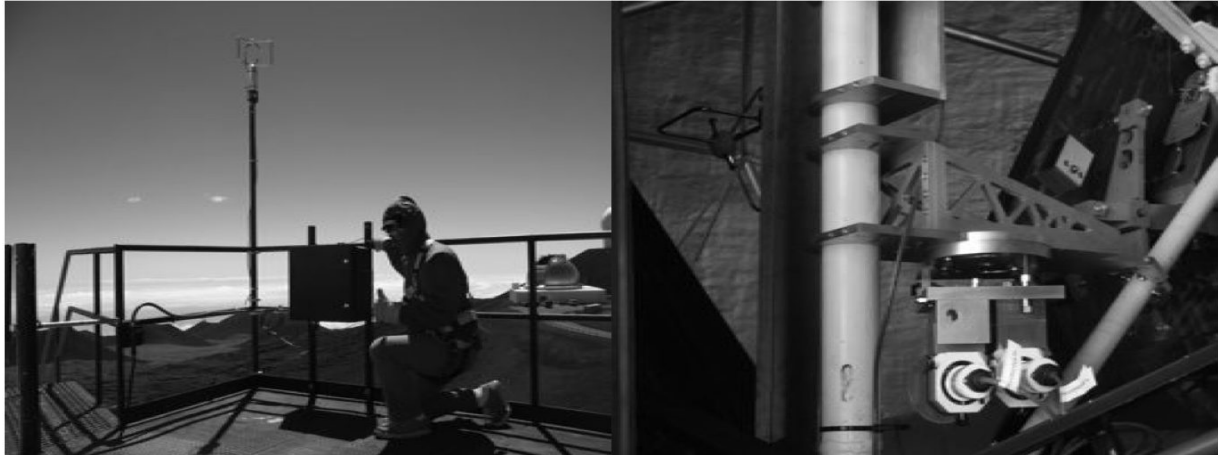
Figure 7. Left: Sonic anemometer and temperature sensor installed on Keck 2 dome top. Right: Scintillometer transmitter and receiver installed alongside the Keck 2 primary mirror.
