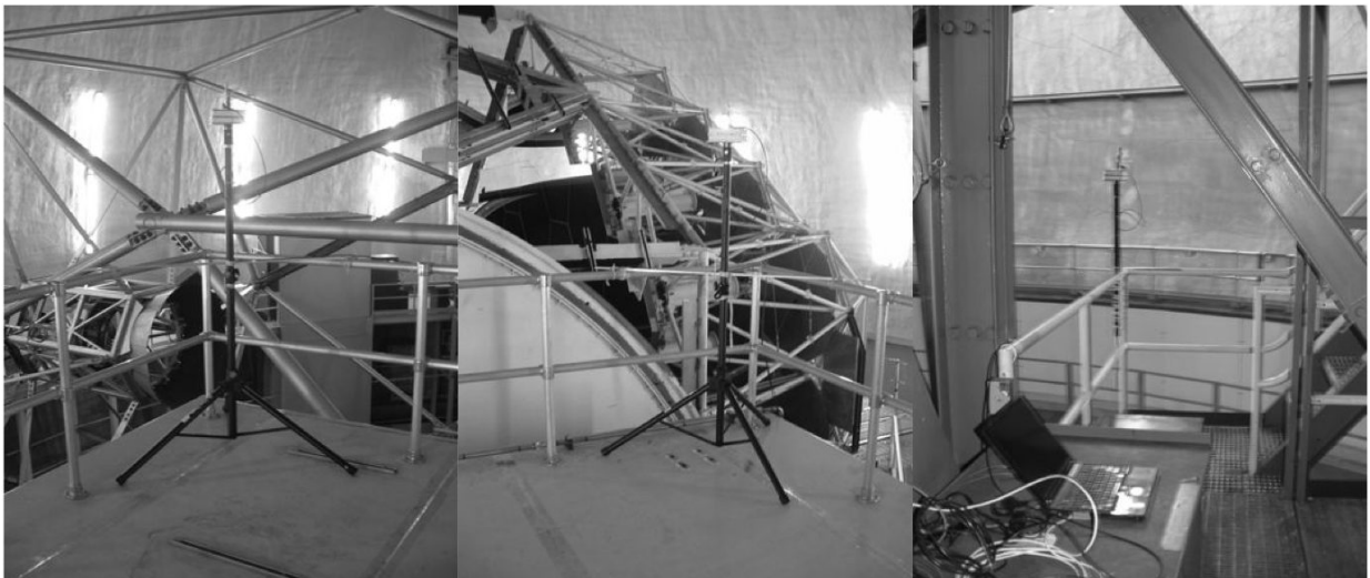
Figure 3. Acoustic sensors at the Keck 1 telescope, left and middle are views of the top of the AO enclosure, right is down below the elevation axis to the rear of the telescope. During science observations two sensors were in front of the mirror plane, one sensor was behind.
