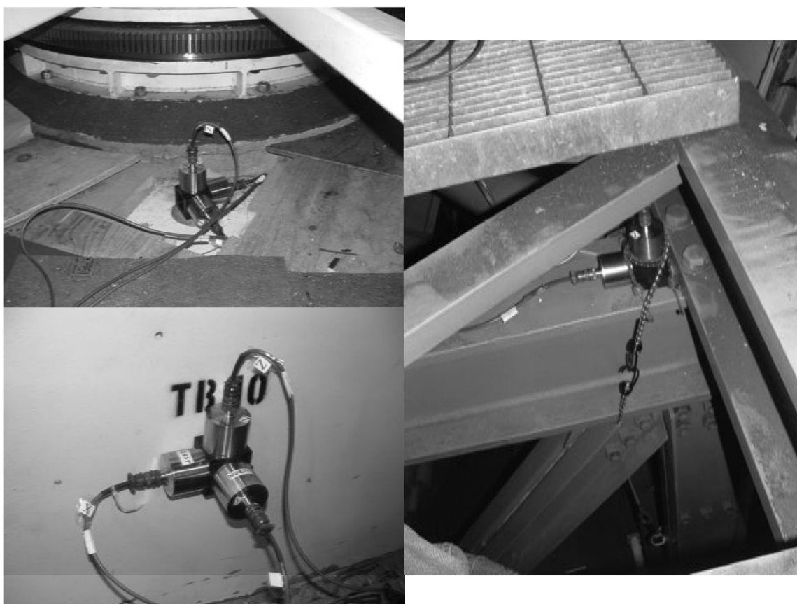
Figure 5. Views of the 3D accelerometer sensor on the Nasmyth platform supports, on the pier and next to the pintle bearing.
