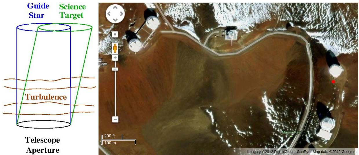
Figure 1. Anisoplanatism in a Natural Guide Star Adaptive Optics System and the Siting of the MASS/DIMM on Mauna Kea. On the left is shown the columns of turbulence sampled by the guide star (blue) and a science target (green). Due to the vertical extent of atmospheric turbulence, light from the guide star and light from the science target encounter different columns of atmospheric turbulence, yielding a difference in the phase aberrations between the wavefronts. This is the effect of angular anisoplanatism. The effect depends on both the time-dependent vertical distribution of atmospheric turbulence and on angular offset from the guide star. Measurements of the vertical turbulence profile C_n^2(z) may be performed using a MASS/DIMM unit currently in operation on Mauna Kea. The unit is located near the Canada France Hawaii Telescope, as indicated by the red dot in the image.
