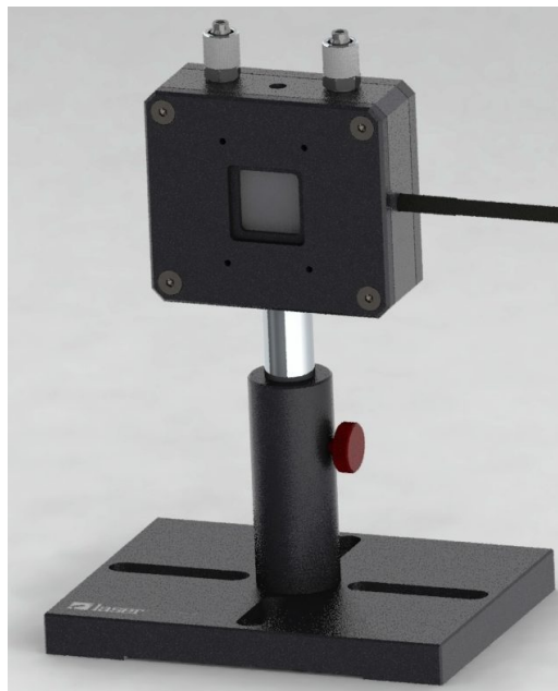
Fig. 2 Picture of the complete detector head, showing the detector mounted onto the water-cooled heat-sink.
