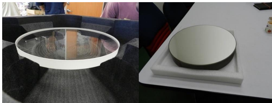
Figure 3. The left panel shows the Schmidt plate fabricated by Nikon Corporation. The right panel shows the spherical mirror fabricated by Control Optics Taiwan Inc.
