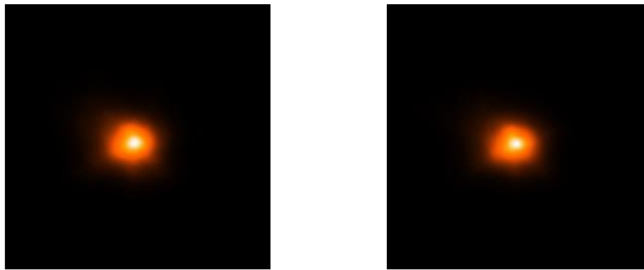
Figure 2. As-built PSF for field center (left) and field edge (right) of the PFS metrology camera after considering all degradation factors.
