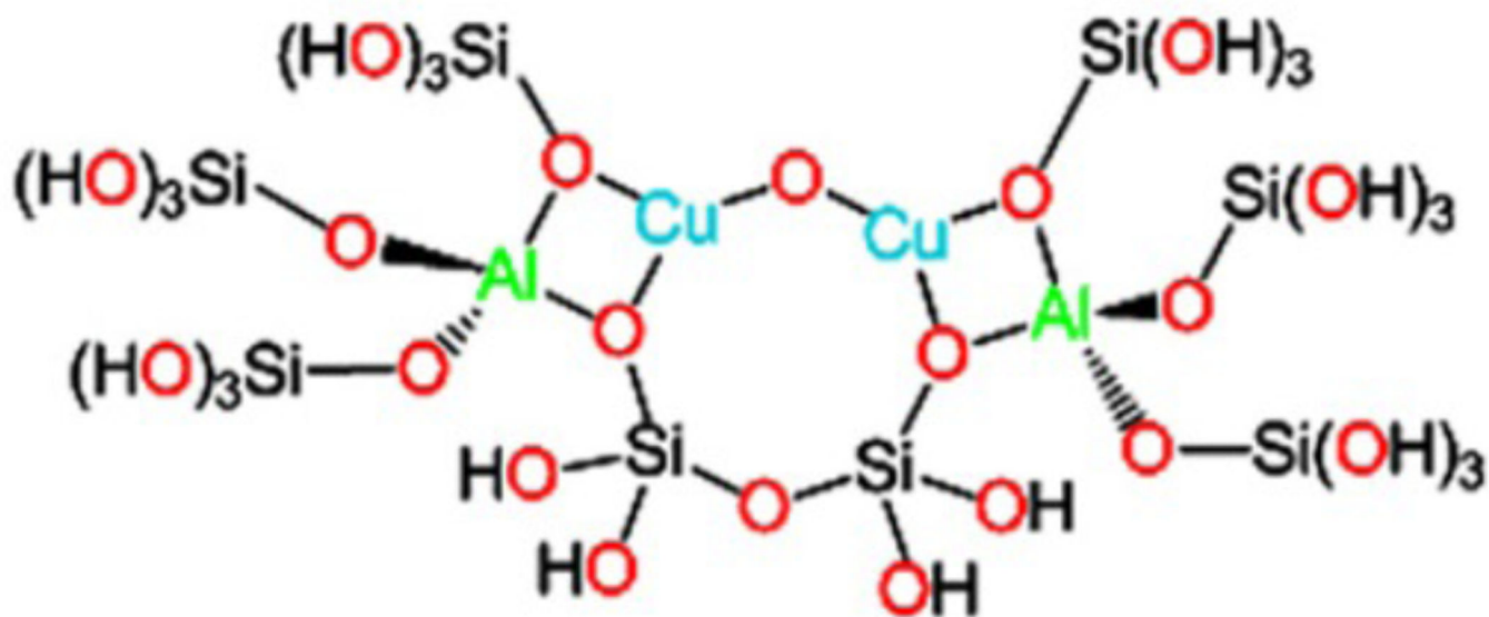
Figure 131. Model of the active [\text{Cu}_2\text{O}]^{2+} core in the 10-membered ring of the ZSM-5 lattice. (Reprinted with permission from Ref. 39 .)
