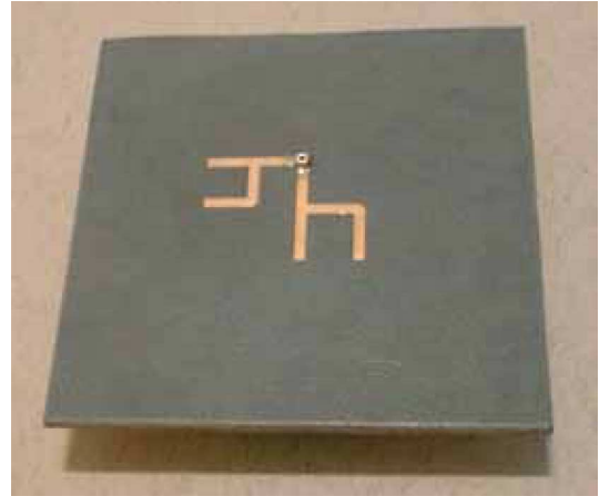
Fig. 10. Final antenna layout fabricated on RT/Duroid 5880.
