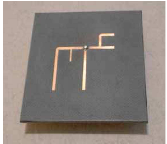
Fig. 6. Boolean PSO-designed antenna element fabricated on RT-Durroid 5880.
