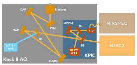
Figure 2. Conceptual layout of KPIC, as integrated on the Keck II AO bench, and feeding IR workhorse camera NIRC2, and high-resolution IR spectrograph NIRSPEC, by means of a fiber injection unit (FIU).
