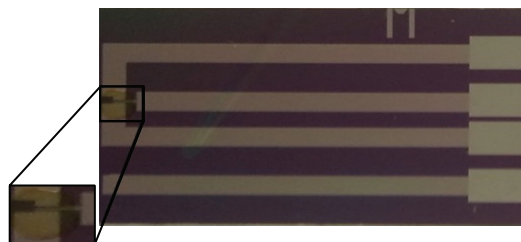
FIGURE 16: Glucose sensor after functionalization.
