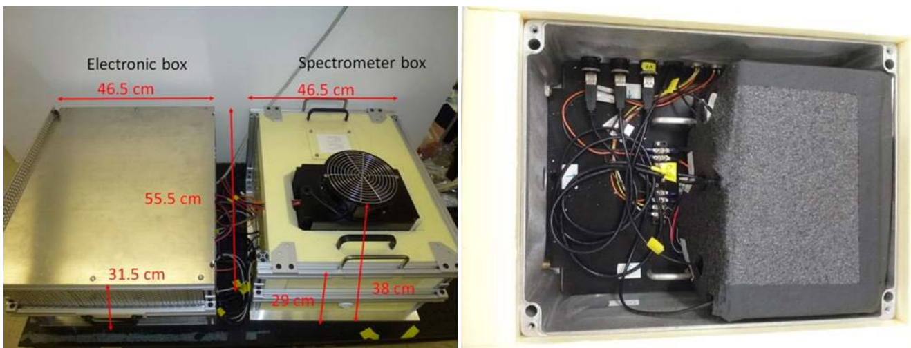
Figure 5: Left : Spectrometer System. Thermally stable Spectrometer box with the Peltier cooler sticking out, next to the electronic box (computer, etc). Right : opened Spectrometer Box on the right panel (2 QE Pro + 1 Flame spectrometer located under the black insulation).
