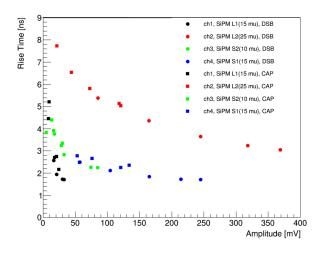
Figure 1. Rise time of the pulses as a function of the amplitude for the four different SiPMs. The data recorded with the plastic fibers and the quartz capillaries are distinguished as dots and squares. For each of the two data sets with plastic fibers and capillaries there are 5 measurements corresponding to beam energies of 20, 50, 100, 150 and 200 GeV.
