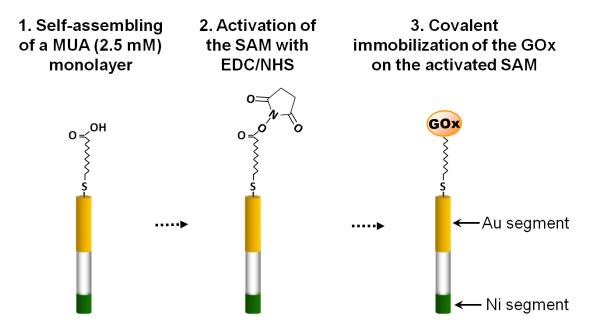
SI Figure 1. Schematic representation of the surface chemistry involved in the magnetic swimmer modification with GOx.
