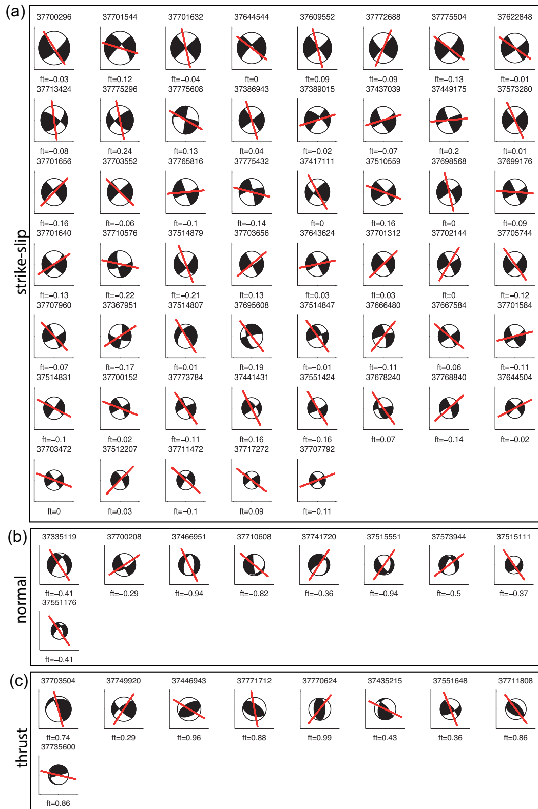
Figure 12. Comparison of FinDer-determined rupture strike (red line) and focal mechanisms/moment tensor solutions for the real-time detected earthquakes ( 2.2 \leq M \leq 5.1 ) shown in Fig. 11. The size of the beachballs scales with magnitude. We apply a rake-based classification of faulting style (Shearer et al. 2006) that produces output values ft from -1 to 1 . For most events, the FinDer-determined rupture strike and the strike of one nodal plane of the corresponding focal mechanism agree to within \pm 25^\circ . Errors are smallest for the strike slip ( -0.25 \leq ft \leq -0.25 ) earthquakes, but strike estimates for many normal ( ft < -0.25 ) and thrust ( ft > 0.25 ) events are reasonable.
