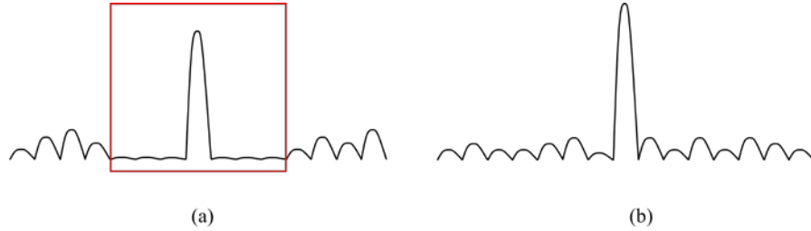
Fig. 1. Illustration of focusing light to a target location by (a) the transmission matrix inversion method, and (b) the phase conjugation method. The red box in (a) denotes the selected field of view.
