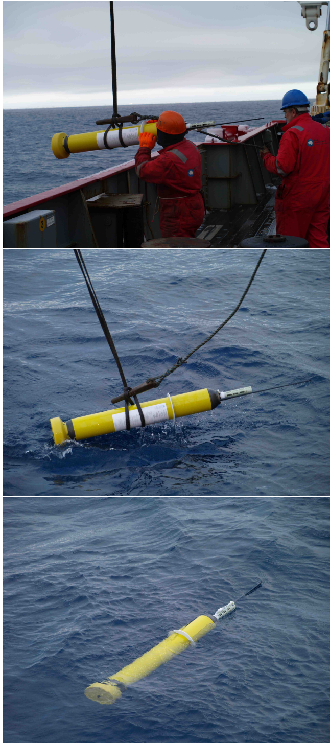
Figure 26: (a) Argo float carried over the side of the JCR using the winch. (b) Argo float just before release. The metal bar is pulled out quickly releasing the rope knot. (c) Argo float immediately after deployment. All floats remained in a horizontal position as the JCR steamed away. This occurred because new floats have smaller holes to minimize sediment intake and thus take longer to fill with water and flip up vertically.
