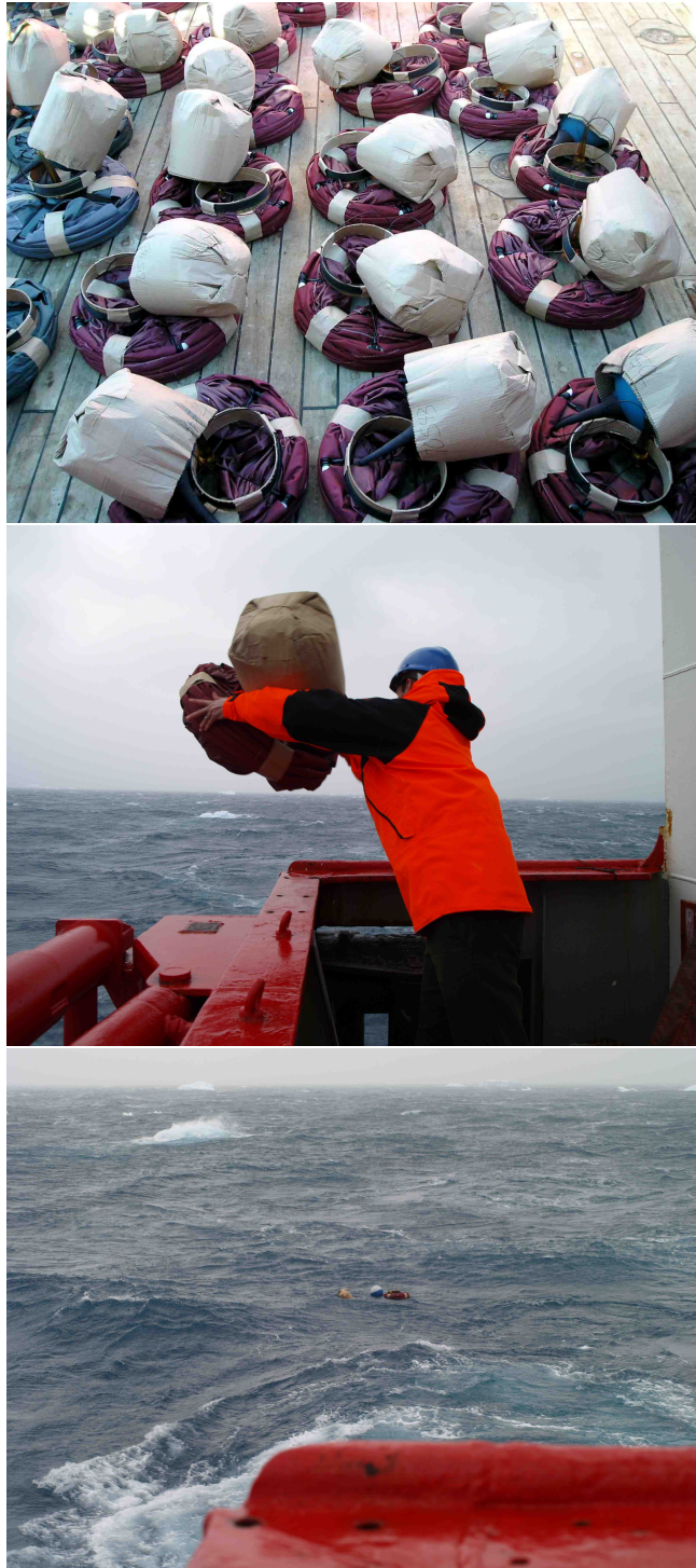
Figure 22: (a) Drifters on the back deck after having been activated by removing the magnet on the buoy. (b) Drifter deployment off the stern of the JCR. (c) Drifter floating in the water shortly after deployment. The cardboard hood covering the buoy has fallen off, but the cardboard bands can take hours to dissolve.
