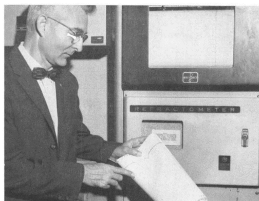
CHECK. Dow's John C. Moore checks chromatogram obtained by gel permeation chromatography, which separates a polymer's constituents by molecular weight
