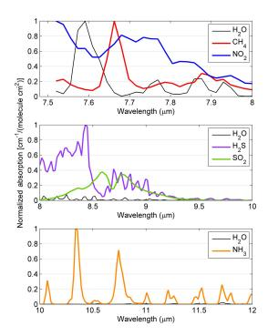
**Figure 5.** Normalized absorption spectra of  $H_2O$ ,  $CH_4$ ,  $NO_2$ ,  $H_2S$ ,  $SO_2$ , and  $NH_3$  extracted from the HITRAN 2012 database and convolved to the HyTES spectral response functions displayed in different wavelength ranges in the thermal infrared from 7.4 to  $12 \,\mu$ m.
