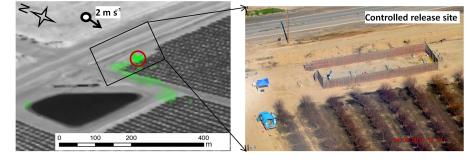
**Figure 10.** Example of HyTES-detected methane (green) with overlay on grayscale surface temperature (left) at the natural gas controlled release site (inset photograph). Detected methane in the HyTES image is displayed in green with the higher intensity color corresponding with highest concentration of methane at the release point circled in red.
