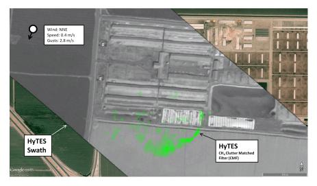
**Figure 9.** HyTES-detected methane plumes over a dairy farm in the San Joaquin Valley, California, during February 2015 displayed in Google Earth with the methane plume in green overlayed on HyTES grayscale surface temperature retrieval. The dispersion of the detected plume is consistent with wind measurements in the local area (from NNE at  $0.4 \text{ m s}^{-1}$  with gusts to  $2.8 \text{ m s}^{-1}$ ).
