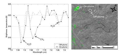
**Figure 8.** HyTES brightness temperature spectra (left) from 7.5 to 8  $\mu$ m for an on-plume and off-plume pixel indicated in the CMF temperature overlay (right) for a plume over the Kern River oil field in July 2014. The presence of H<sub>2</sub>O features in both the on-plume and off-plume pixels but only CH<sub>4</sub> in the on-plume pixel indicates the latter detection is not a false positive.
