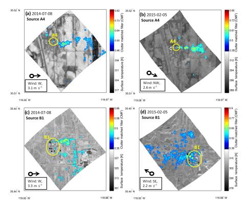
**Figure 7.** Examples of persistent methane plumes detected by HyTES over oil condensate storage tanks in the Kern Front and Kern River oil fields near Bakersfield, California. Sources A4 in panels (**a**) and (**b**), and B1 in panels (**c**) and (**d**) were detected during July 2014 and February 2015. Plume enhancements are shown in color using the CMF method overlayed on a surface temperature image.
