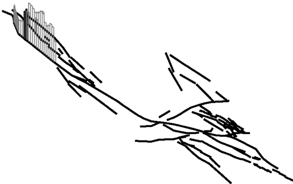
Fig. 3. Example of a large event on the northern San Andreas fault in a model of type II, in which all faults have the property of dynamic fracture weakening. The epicentral segment is shown in dark. Note that slip in this event occurs not only on the San Andreas fault proper, but also on other sub-parallel faults, demonstrating that earthquakes in the simulations are non-compact events. Maximum slip in this event is 11.04 m.
