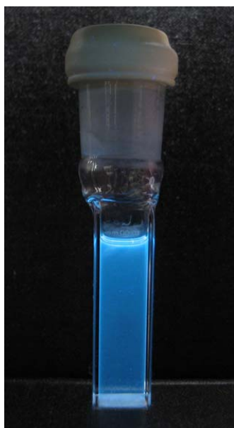
Figure S-3. Photograph showing the fluorescence of HPI-Ac solution after degassing by Argon gas purging. The cuvette was specially designed for efficient gas purging.
