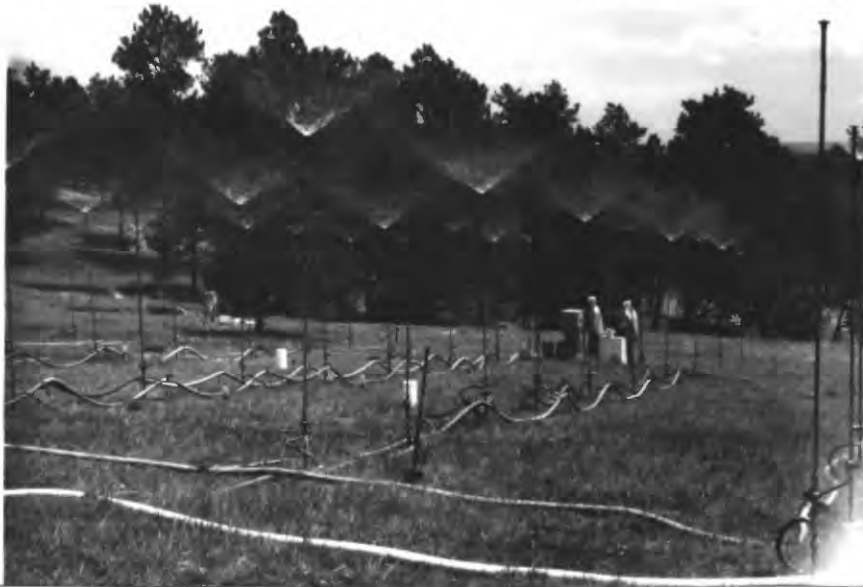
Figure 4.--Rainfall simulator in operation, plot 2, Willow Gulch study watershed.
