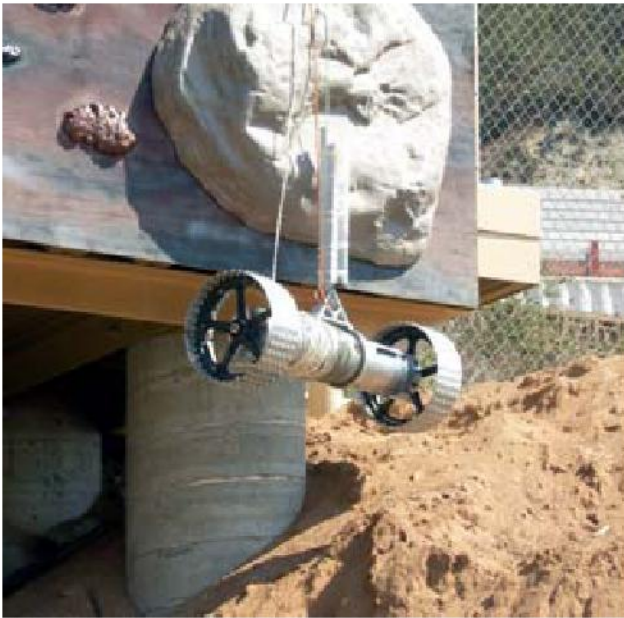
Figure 7—Axel lowered over a simulated promontory mounted on the viewing platform in the JPL Mars Yard.
