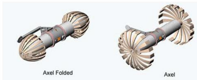
Figure 6—The Axel rover folded in its launch configuration (left), unfolded for surface deployment (right)
