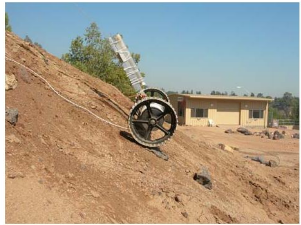
Figure 8—The Axel rover prototype driving down a 40° slope.
