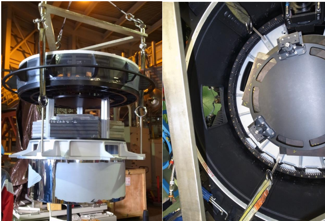
Figure 2. The structure used in the PFI fitting tests (left) and PFI installed inside POpt2 without the cable wrapper (right).
