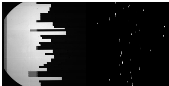
Video 3. CSU_open_mask (left) and CSU_mask_change (right) are two videos that show common mask reconfigurations. The open mask shows the bar movements from an open configuration that was used for imaging to a mask configuration. The mask change video shows the bar motions when observers switch from one mask to a second mask. http://dx.doi.org/2doi.number.goes.here & http://dx.doi.org/2doi.number.goes.here .
