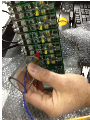
Figure 10. Image of the amplifier board being tested with a power resistor that was used to heat individual components. Board components were individually heated and cooled to isolate where the thermal dependency was located.
