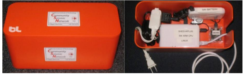
Fig. 1 – CSN instrumentation showing MEMS accelerometer, onboard computer and backup battery.
