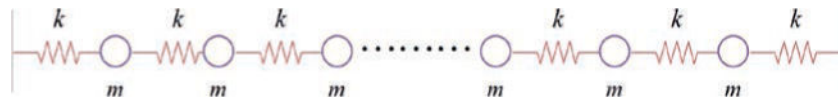
Figure 1. The spring-mass model. The black dots denote continuation of springs and masses.
