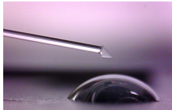
Fig. 8 Probe assembly process. Video 1 shows the process by which a small portion of UV epoxy is applied to the bottom surface of the \mu -prism. (Video 1, MP4, 24.2 MB) [URL: http://dx.doi.org/10.1117/1.NPh.4.1.011002.1 .]
